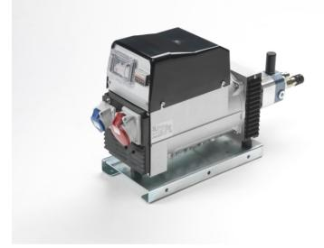
HW series are professional **DC** welders with capacity of 170 - 200 Ampere powered by hydraulic gear motor. The tools can be connected to the circuits of earth moving equipment, trucks, cranes, mobile workshops and all machines with sufficient hydraulic capacity.
